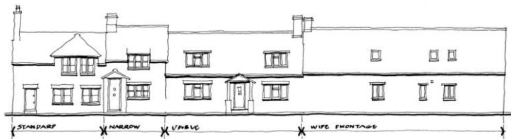
Four cottages | A continuous building line and consistent use of natural stone unifies this group of differing architectural styles. The informal rhythm of the elevations results from a variety in plot widths (North Lane).
